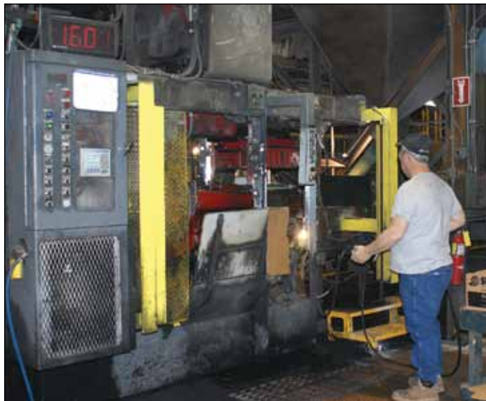
Bremen Castings Inc. installed a second automatic molding line in 2003, which increased capacity and mold cooling time.
